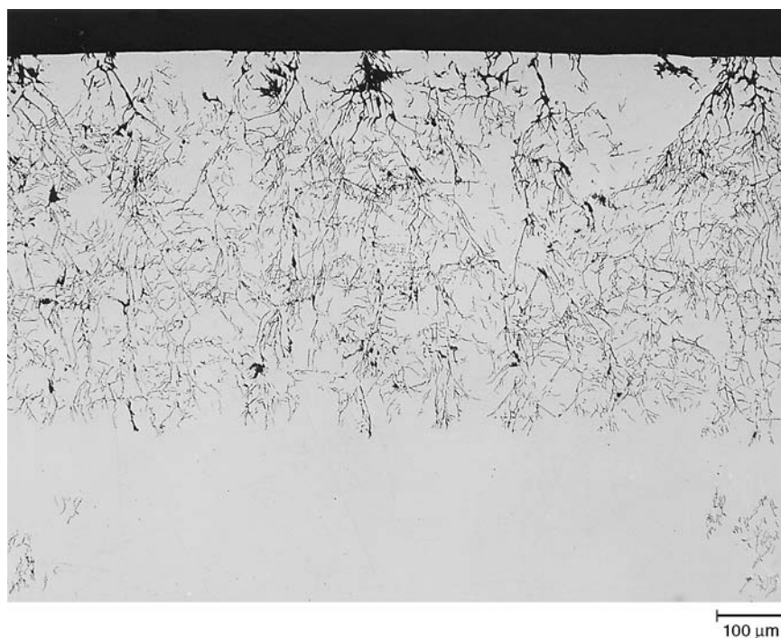
Fig. 24 Stress-corrosion cracking of C-276 alloy in HF solution
