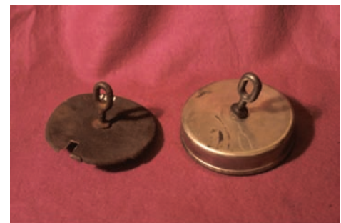
Fig. 4 An aerosol can burst unexpectedly when the owner tried to clean off external rust that had developed over several years' storage inside a bathroom cabinet. The cross section of the joint at the bottom of the can revealed that the product side of the can was not a factor. All the wastage was from the outside of the can. The bottom thin coating had been locally eroded, leaving the can bottom exposed to localized corrosion as moisture and deposits accumulated with time. Attack was enhanced by condensation and evaporation cycles in the bathroom cabinet. The can base was completely penetrated at the time the user attempted to clean away the rust from the can. Control: The can should have been discarded based on its obvious deteriorated condition.
