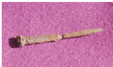
Corrosion form and mechanism Atmospheric, crevice corrosion Material Steel Product form Nail
