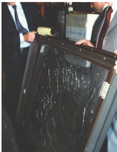
Corrosion form and mechanism Environmental crazing, stress-corrosion cracking Material Polycarbonate Product form Window
