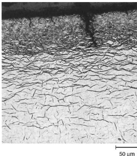
Fig. 7 Micrograph of severely hydrided unalloyed titanium. Original magnification approximately 200 \times
