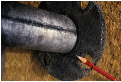
Corrosion form and mechanism Metallurgically influenced corrosion, intergranular (end-grain attack) Material Type 304 stainless steel Product form Flange
