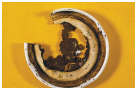
Corrosion form and mechanism Uniform corrosion, atmospheric Material Ferrous metal, carbon steel Product form Pickle jar lid
