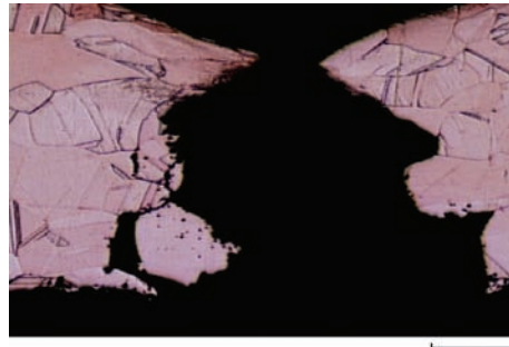
Corrosion form and mechanism Metallurgically influenced corrosion, intergranular attack Material Copper Product form Pipe for fuel oil
