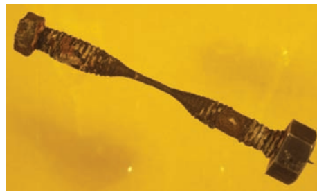
Corrosion form and mechanism Aqueous corrosion, crevice corrosion, galvanic corrosion Material Carbon steel bolt with stainless steel nut Product form Bolted fastener
