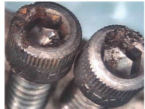
Corrosion form and mechanism Localized pitting, microbiologically influenced corrosion (MIC) Material Steel Product form Allen-head bolts
