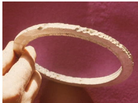
Corrosion form and mechanism Stray-current corrosion Material Type 304 stainless steel Product form Flange spacer
