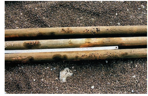
Corrosion form and mechanism Mechanically assisted degradation, impingement Material Copper Product form Pipes from chiller unit
