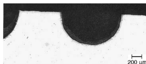
Fig. 29 Pitting attack in alloy 601
