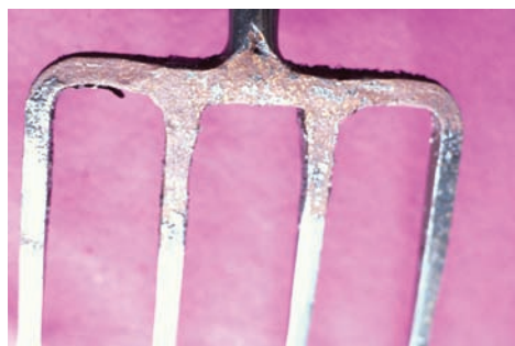
Corrosion form and mechanism Uniform corrosion, atmospheric, filiform Material Type 420 stainless steel Product form Pitchfork
