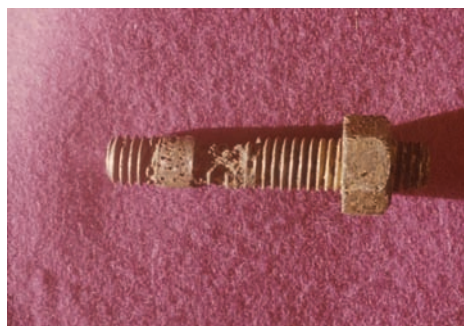
Corrosion form and mechanism Crevice corrosion Material Ni-Cr-Mo alloy Product form Retainer bolt
