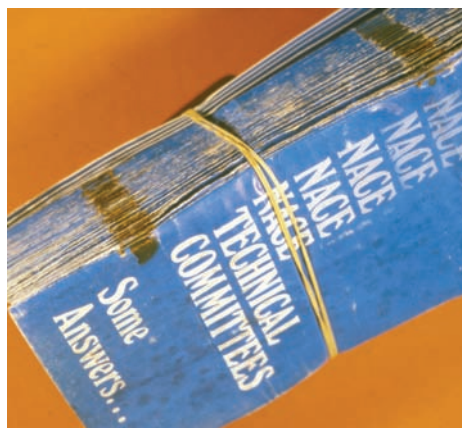
Corrosion form and mechanism Uniform corrosion, atmospheric Material Carbon steel Product form Paper staples
