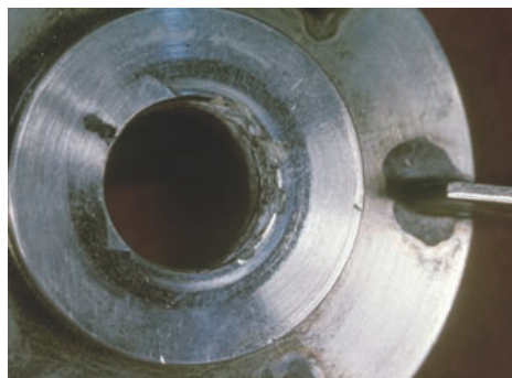
Corrosion form and mechanism Metallurgically influenced corrosion, galvanic corrosion, crevice corrosion Material Stainless steel, carbon steel Product form Stirrer
