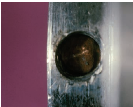
Corrosion form and mechanism Metallurgically influenced corrosion, galvanic corrosion, crevice corrosion Material Stainless steel, carbon steel Product form Stirrer
